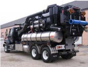
We accepted delivery of our new Sewer Vac-All truck, which replaces our old “Blue Goose” which was on its last legs. This truck will tremendously improve our ability to clean and maintain our old sewer lines.
